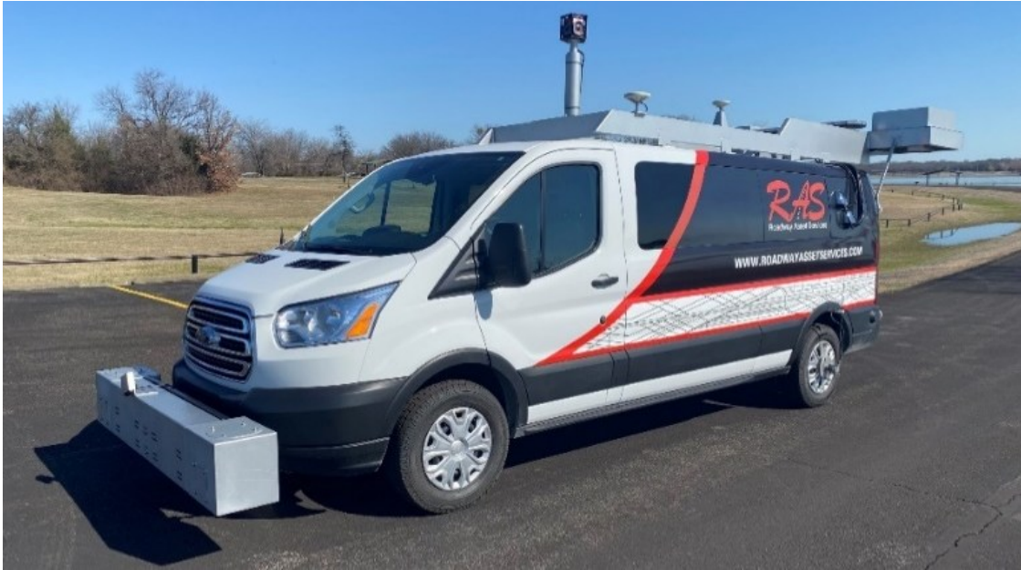
RAC Survey Vehicle (Version 1) with LCMS-2 and Ladybug 5+ Camera
