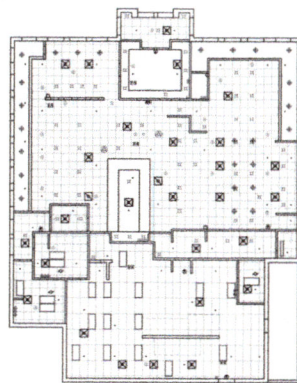
4 Reflected Ceiling Plan Scale: 1/16" = 1'-0" ( AREA: 6,600 SQ. FT. )
